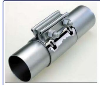
Inner sleeve provides a tight seal with the patented dual tongue-&-groove feature.
